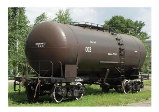
Is intended for transportation of viscous oil products by railways with gauges 1435 mm or 1520 mm. It has frame without side belts, internal system of tank vapour heating, side discharging valve controlled from the top, strengthened tank design. Brakes – automatic pneumatic, manual parking. Running gear – two double-axle bogies mod.18-10 type 2 (GOST 9246-2004). 0 Automatic coupler CA-3. The draft friction gear of increased power consumption of class, not lower than T3
