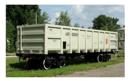
The open-top car is universal four-axle, all-metal freight car with welded body and semi-cylindrical bottom intended for transportation of timber, rolled steel, loose packaged, piece loads requiring no protection from atmospheric precipitation. The car body is without discharging hatches with rounded surfaces in jointing corners between the under frame, side and end walls, and insures tilter unloading with possible minimum load remaining.
