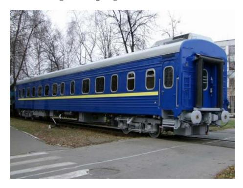
Passenger sleeping coach of locomotive traction is intended for passenger transportation by railways of Ukraine, the CIS and Baltic countries with 1520 mm gauge for motion speed up to 160 km/h.
