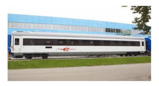
Passenger compartment coaches of locomotive traction are intended for passenger transportation, including disabled (mod.61-778 AI) by railways of Ukraine, the CIS and Baltic countries with 1520 mm gauge for motion speed up to 160 km/h.
