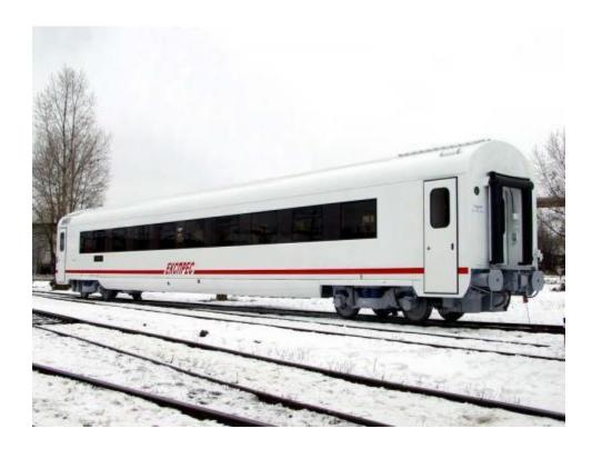
Passenger coach with sitting places of locomotive traction. It is intended for passenger transportation by railways of Ukraine, the CIS and Baltic countries with 1520 mm gauge for motion speed up to  $160 \, \text{km/h}$ .
